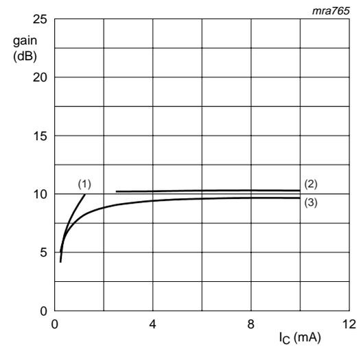
$V_{CE} = 6 \text{ V}; f = 2 \text{ GHz}.$
