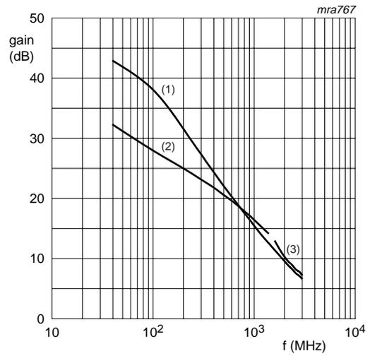
$V_{CE} = 6 \text{ V}; I_C = 5 \text{ mA}.$
